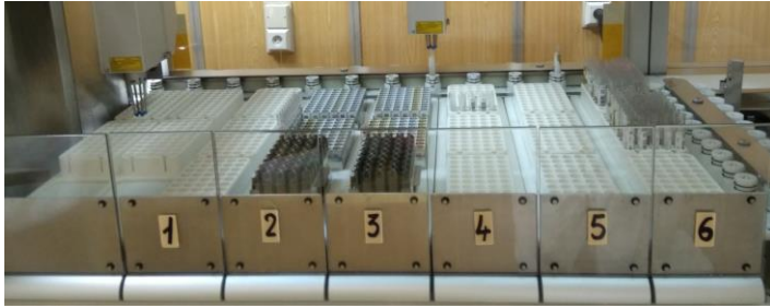
Figure 6 AutoMate Automatic sorting line The individual racks in the sorting line (numbered 1 - 5) hold samples directed to the different analysers, or samples that have already been analysed and are destined for archiving in the refrigerated room (number 6). On the left and in the back centre we can see the moving arms that sort the samples.
