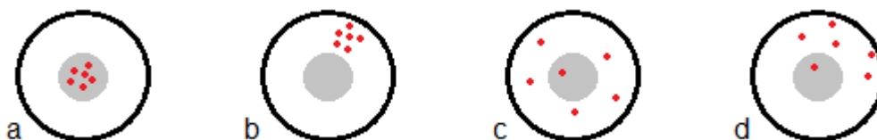
Figure 30 Relationship between accuracy, precision and trueness of the laboratory method There are four possibilities for the results' correctness: a - precise true (represented by the shots in the middle circle of the target), b - precise false, c - imprecise individually false, arithmetic mean true, d - imprecise false
