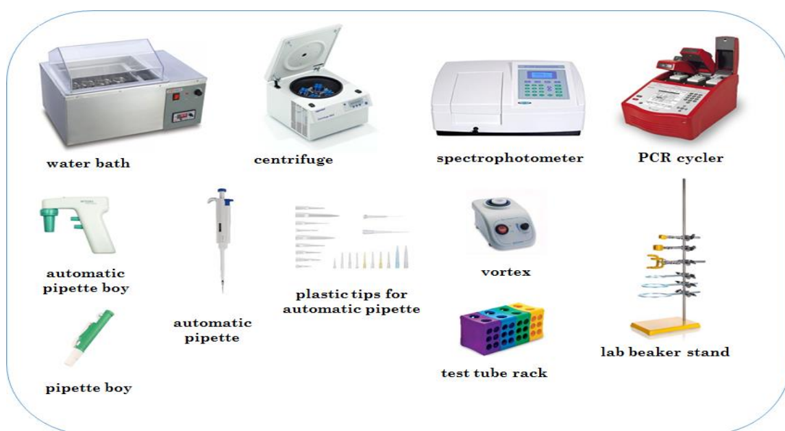
Figure 6: Basic laboratory tools and machines. Many tools are necessary for each experiment. Laboratory practical represents one small experiment. Water bath – used for the incubation of a test tube with reagents (a reaction proceeds at specific temperature). Today, we prefer a dry water bath. Centrifuge – used for separation of liquid reagents or a sediment (solid molecules) from supernatant (liquid reagent above sediment). Spectrophotometer – used to measure absorbance. Polymerase chain reaction (PCR) cycler – a routine machine for amplification of a specific segment of deoxyribonucleic acid (DNA). Automatic pipette boy/pipette boy – used for pipetting with glass pipettes. Automatic pipette – used for pipetting. Vortex – used for mixing reagents. Laboratory beaker stand – used to hold laboratory glass. Test tube rack – used to hold test tubes.
